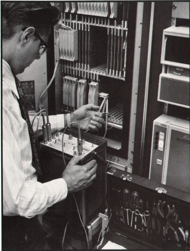
Fig. 14. Light weight, handle, and form factor make the Logic Analyzer suitable for field service applications.
