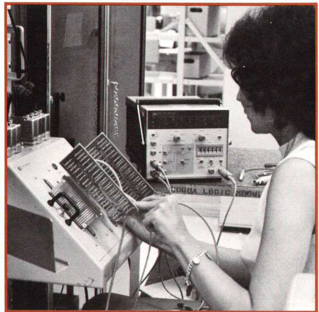
Fig. 6. A \oplus B mode, one of three possible combined-waveform display modes, is useful for comparing test and reference circuit boards in production testing. Only differences are displayed.
